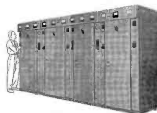
Continental's 317B 50 KW AM broadcast transmitter
